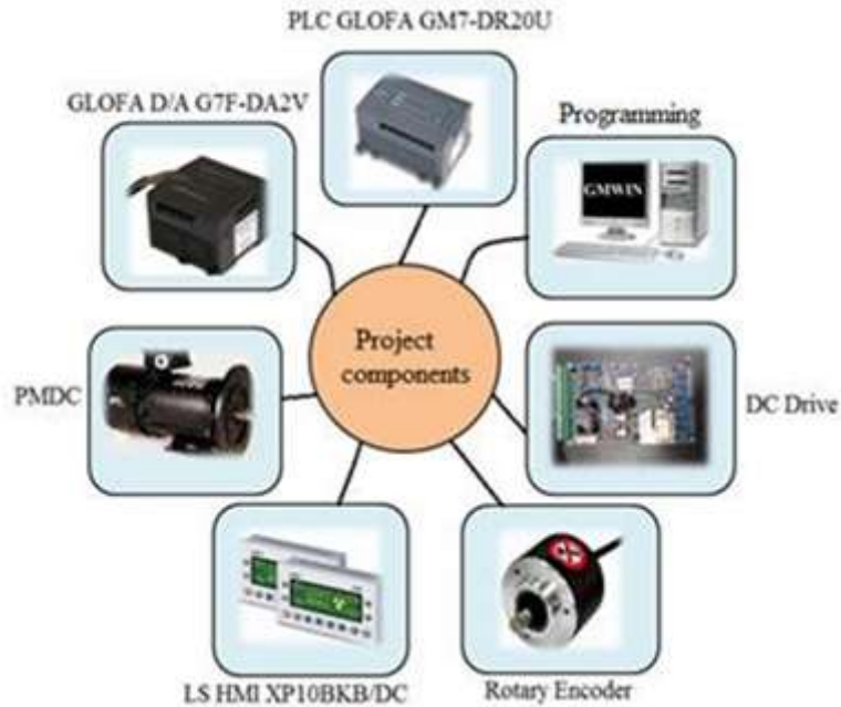
Figure 9 The overall structure of speed controlling DC motor
